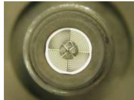
Figure 7. PDE Heat flux sensor utilizing a resistance bridge
