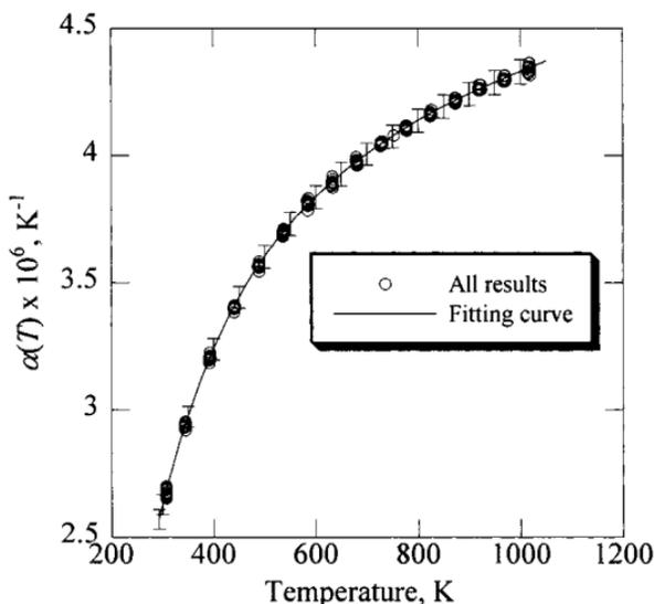
Fig. 2. Linear thermal expansion coefficient,  $\alpha(T)$ , of silicon as a function of temperature.
