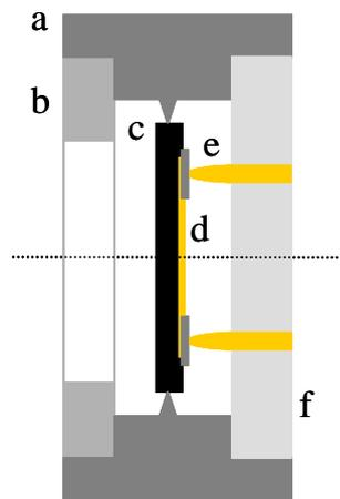
**Figure 3:** Cross section of the specimen holder (a) with diaphragm for shaping the laser pulse (b), specimen, supported by three spikes (c), sputtered gold strip with contact pads made of silver conductive paint (d), spring-loaded contact pin (e) and support for the contact pins made of Teflon® (f).
