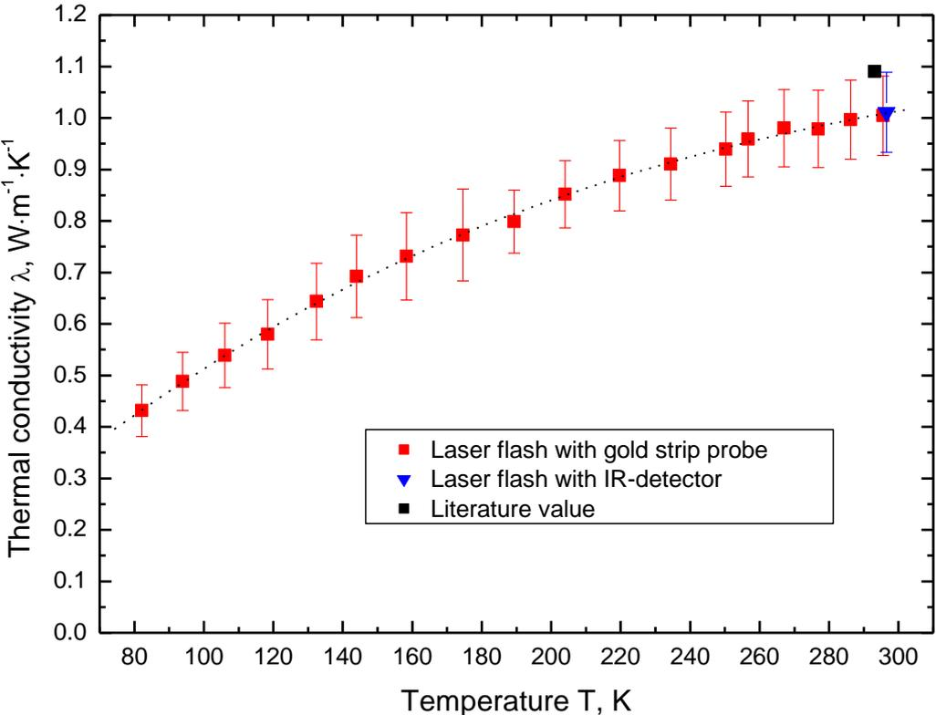
**Figure 9:** Calculated values of thermal conductivity of the investigated BK7 specimen, plotted as function of temperature. For comparison a literature value is also depicted [16]. The dotted line is added as guide to the eye.
