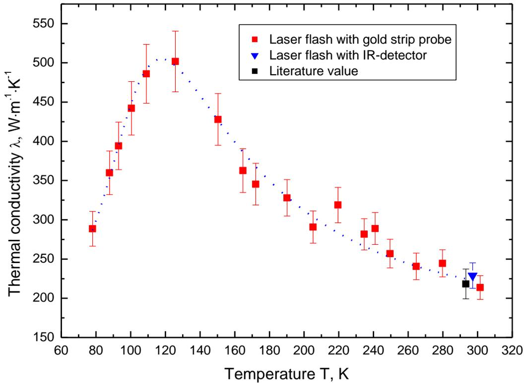
**Figure 10:** Temperature dependence of the calculated thermal conductivity of the polycrystalline aluminium nitride specimen. For comparison a literature value is also depicted [13]. The dotted line is added as guide to the eye.
