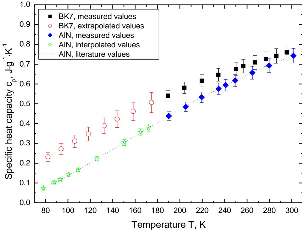
**Figure 8:** Specific heat capacity of the investigated specimens. Depicted are measurement results, the extrapolated values for BK7 and literature data for the specific heat capacity of AlN (Mah et al. [15]).
