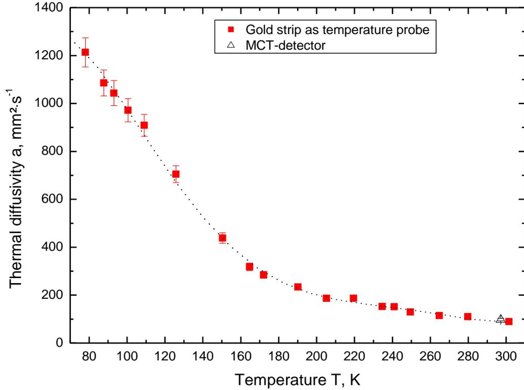
**Figure 7:** Thermal diffusivity of a polycrystalline AlN specimen as a function of temperature, measured by laser flash method. The dotted line is added as guide to the eye.
