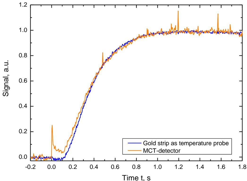
*Figure 5: Comparison of both temperature detection methods using a specimen of BK7 glass at 300 K.*
