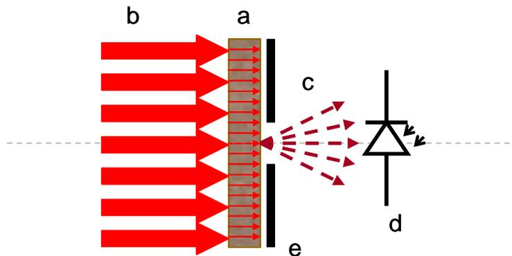
**Figure 1:** Principle of a typical laser flash setup: one side of a disk-shaped specimen (a) is heated with a laser pulse (b). The thermal radiation (c) emitted from the center of the opposite side of the specimen is detected time-dependently with an IR-detector (d) and an optical diaphragm (e).
