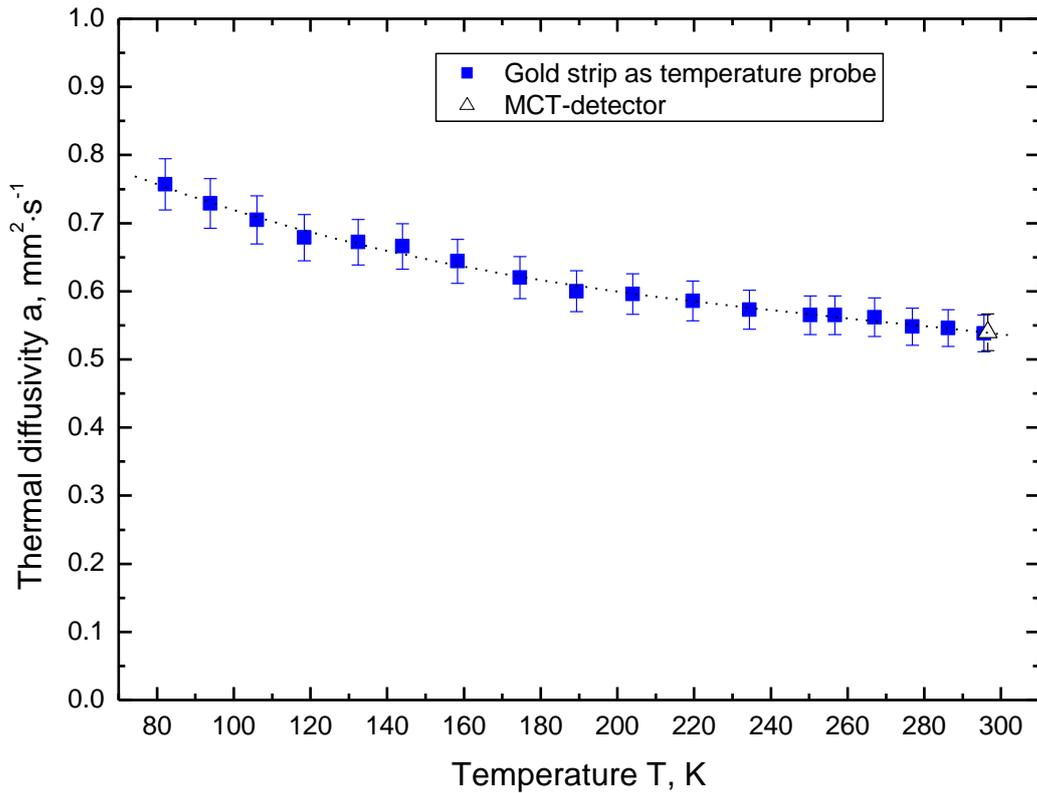
**Figure 6:** Thermal diffusivity of BK7 glass as a function of temperature, measured by laser flash method. The dotted line is added as guide to the eye.
