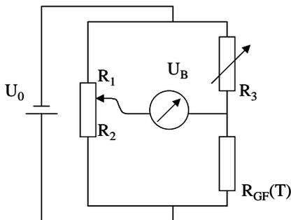
**Figure 4:** Wheatstone bridge circuit for the determination of the temperature-dependent change of  $R_{GF}$ .
