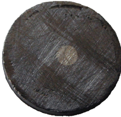
Figure 2: Demonstrator sample made of stainless steel with a silver insert of 2 mm diameter. The diameter of the sample is 12.5 mm.
