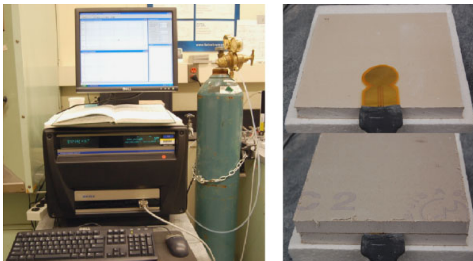
Figure 1. Configuration of a hot disk thermal constants analyzer; a spiral probe placed on the gypsum same is shown in the right.
