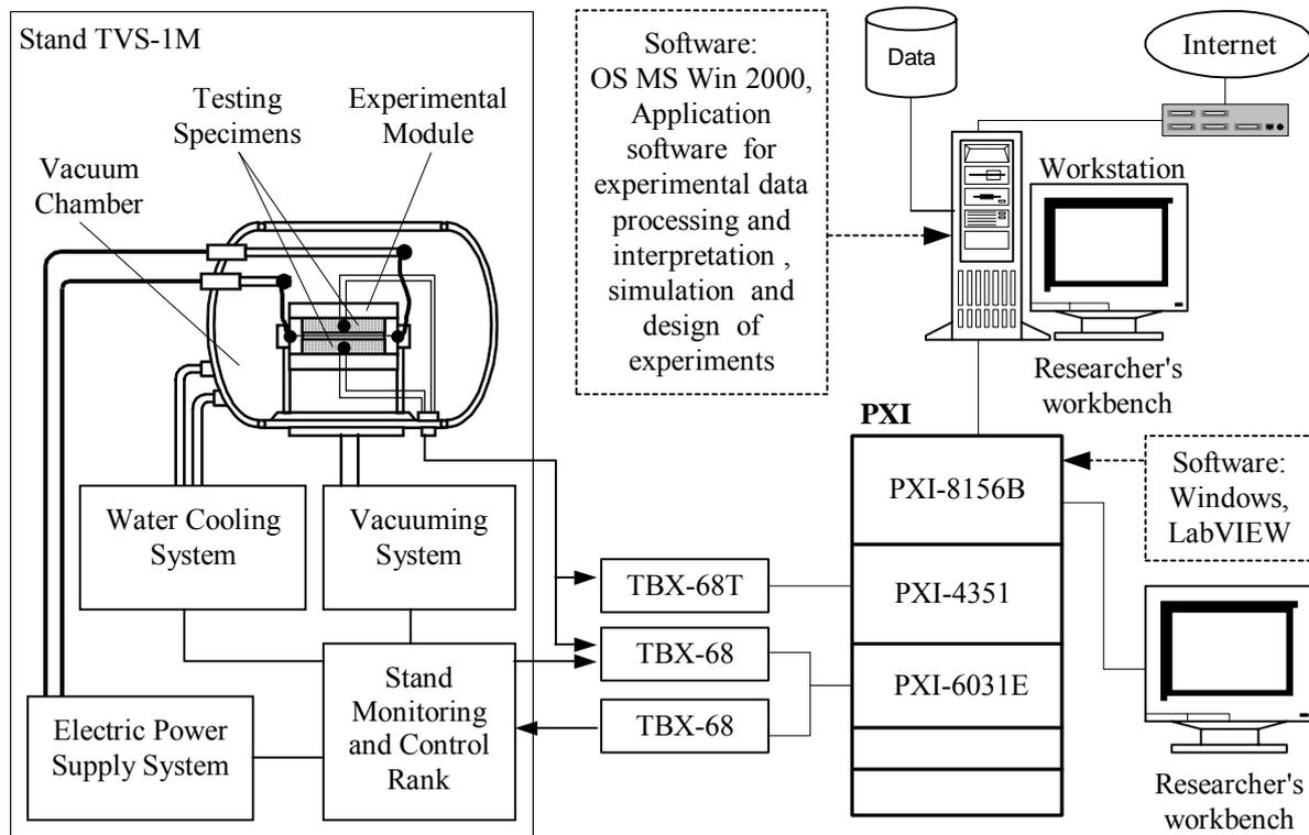
Figure 1. Experimental/computational system configuration.
