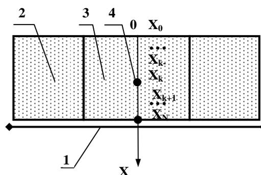
Figure 14. Temperature measurement circuit in specimen: 1 – heating element; 2 – specimen; 3 – specimen's sensing element; 4 – setting points of thermal sensors with coordinates  $X_k$ ,  $k=1, \dots, N$ .
