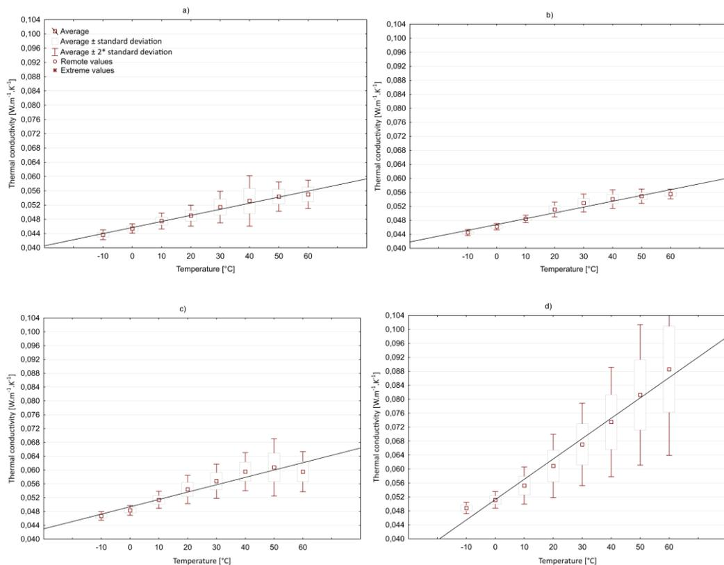
**Fig. 2** Insulation fibreboard thermal conductivity as related to temperature, at different moisture contents of the boards: a) oven dry, b) 2.58%, c) 7.41%, d) 14.29%.
