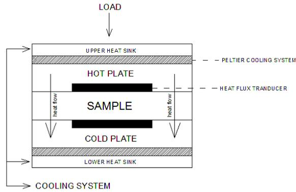
**Fig. 1** Heatflow measurement setup for the tested insulation fibreboards.
