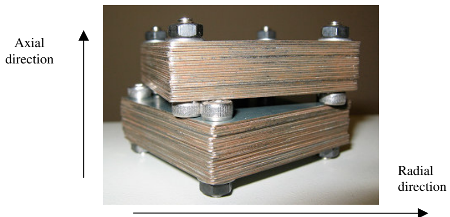
Fig. 1. The stack of metal sheets. By removing the screws it was possible to insert a sensor in between the two sample pieces. A slab measurement was carried out on 2 individual sheets. The arrows give the directions in for the anisotropic measurements.
